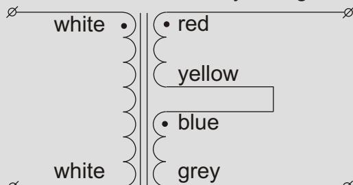
parallel operation to double the secondary current
